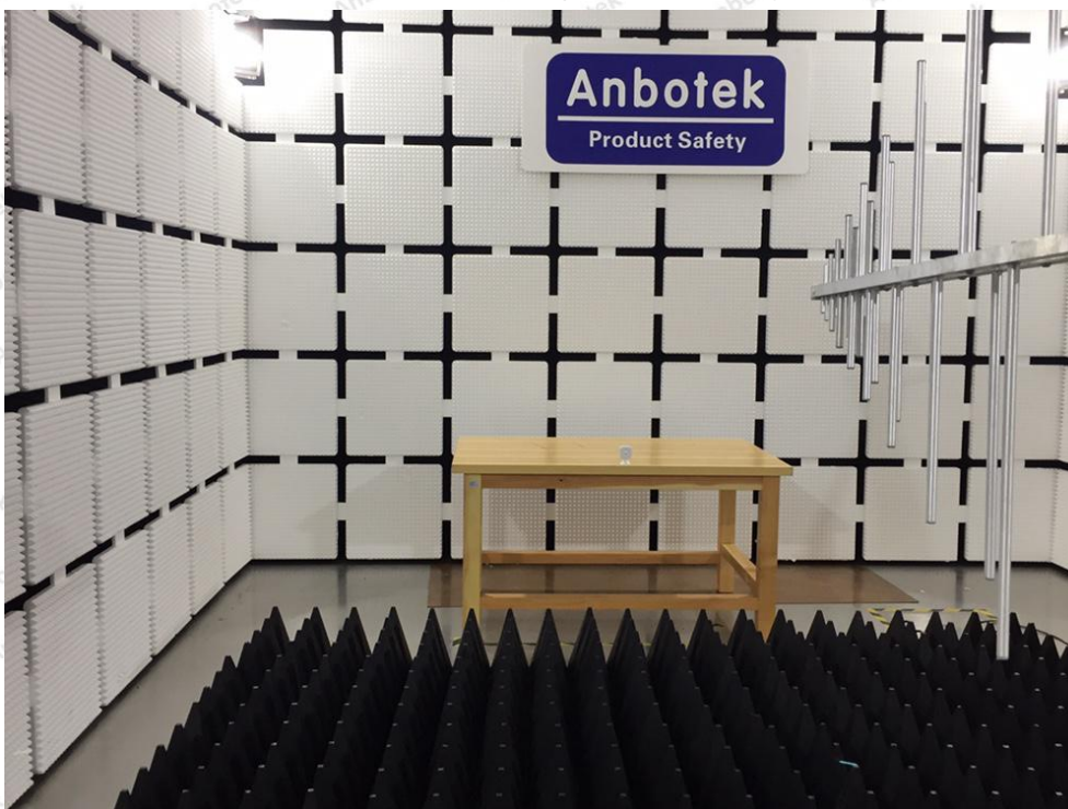
Photo of RF Field Strength Susceptibility Test
